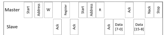
Figure 17. Read Register Operation
