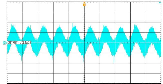
Output voltage (blue) (100 mV/div) Time base : 10 ms/div
