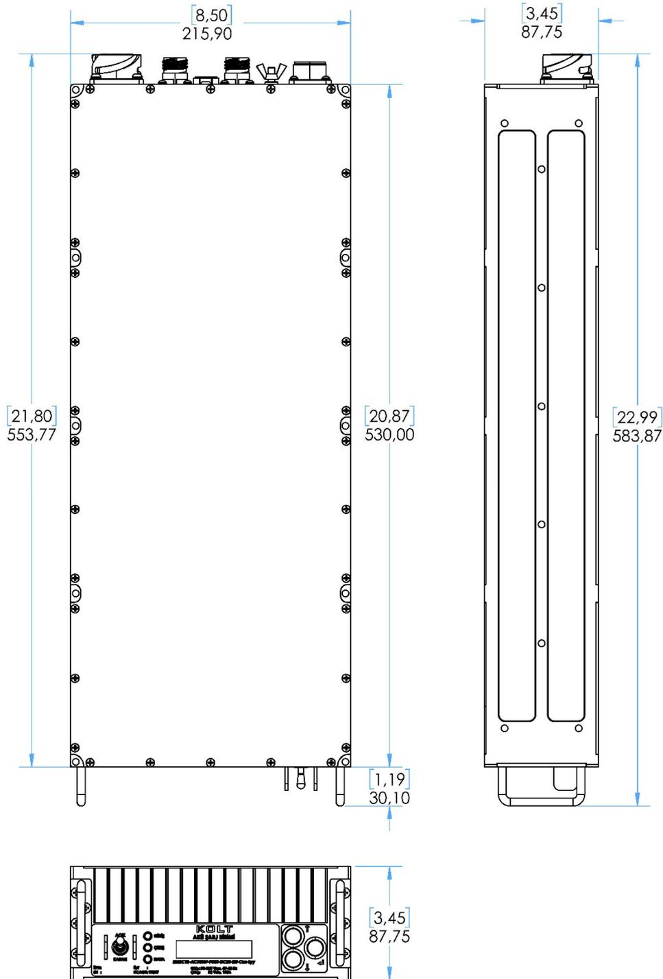
Figure 27. Mechanical Dimensions
