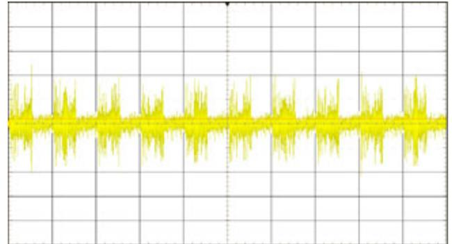
Leakage current (yellow) (10 mA/div) Time base : 20 ms/div
