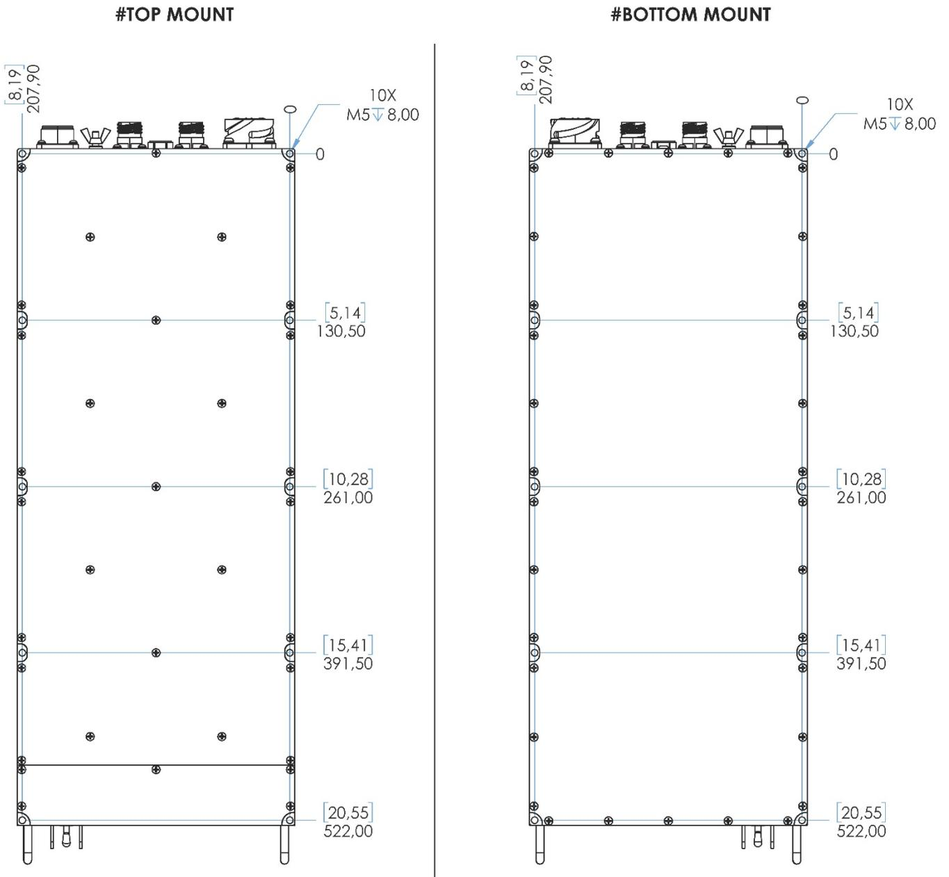
Figure 28. Mounting Details and Mounting Holes Coordinates
