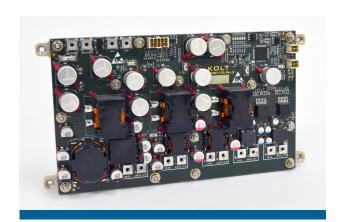
GDK1006 is a 550W DC/DC PoL Converter that operates at nominal 28 Vdc input and generates different output voltage. The cooling plate on this converter includes a mounted thermal pad.
