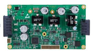
GDK2001 Non-Isolated Bidirectional Power Board is a unit that, when fed with city power line gets fed with (28VDC-32VDC) Input. When supplied from AC / DC converter, it charges the batteries according to the healthiest smart battery charging protocol. The unit adjusts the percentage zone that these modes will occupy during the charging time according to the battery voltages.
